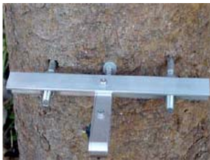
dendrometer typ DR sensor installed
