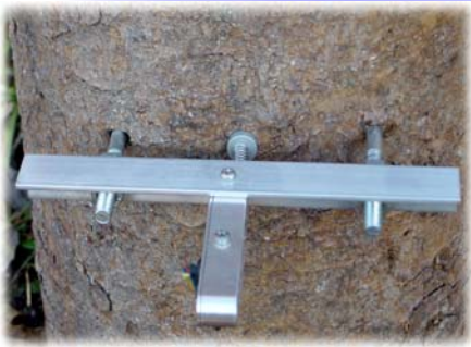
Type DR , for measuring changes in radius, suitable for diameter > 8 cm. The stem is injured by two screws.
