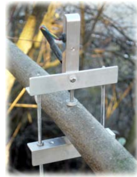
Type DD , the frame can be reduced to meet any size of plant tissue.
