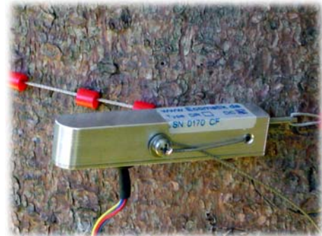
Type DC , For measuring changes in circumference, suitable for diameter > 2 cm, no injury to stem.
