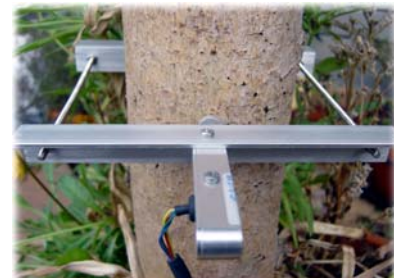
Type DD , for measuring changes in diameter, suitable for diameter < 11 cm, no injury to plant.
