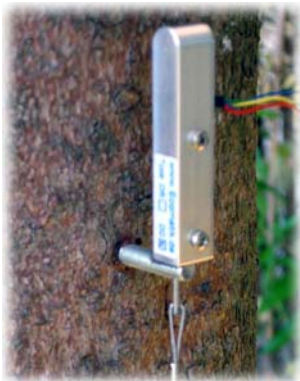
Type DC , very light, the complete sensor is only 16 g (without cable).
