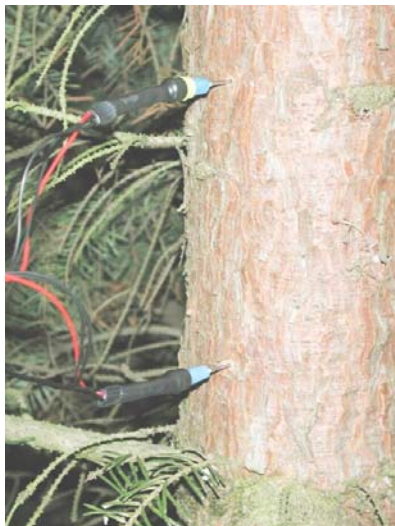
Sapflow sensors installed
